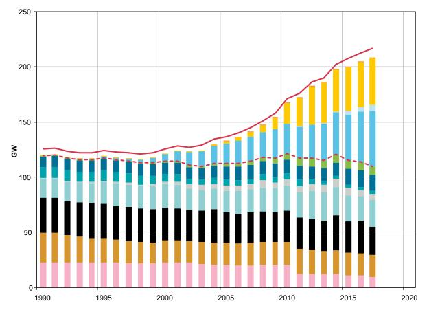
Geothermal Photovoltaics Offshore wind Onshore wind Biomass Hydro (incl. PSH) Petroleum Other fossil Natural gas Hard coal Lignite Nuclear Dispatchable capacity Gross capacity (incl. self-consumption)
