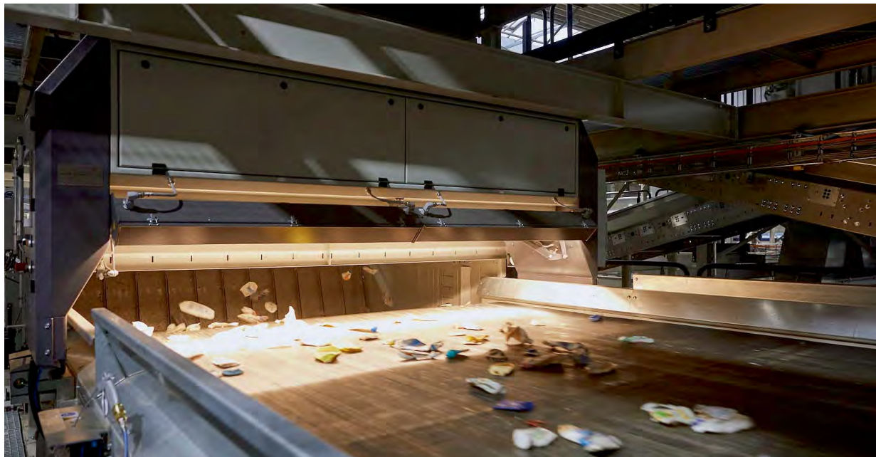
Figure 9: Example of a modern sorting system combining colour and hyperspectral near-infrared sensors (HSI-NIR) 91 ; © REMONDIS
